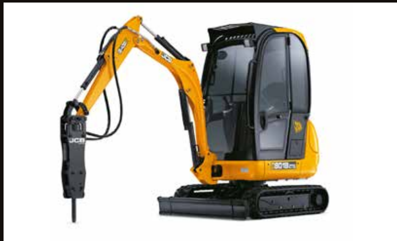
JCB with breaker attachment
